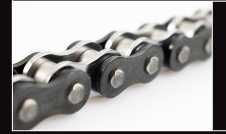
High Grade Steel alloys with the correct heat treatment, advanced precision manufacturing methods and tolerances, customized X-Rings when it's needed and high grade grease make up the quality chain of AFAM.
